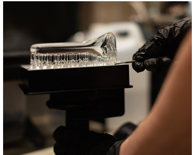
Clear resin 3D prototype on the build platform of the Formlabs Form 3 3D printer
